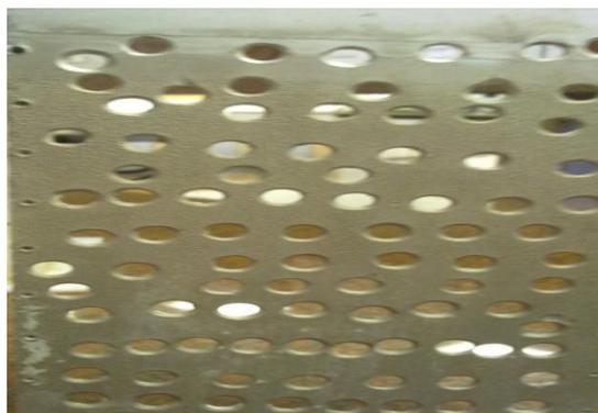
**Figure(3)** perforated aluminum sheet
